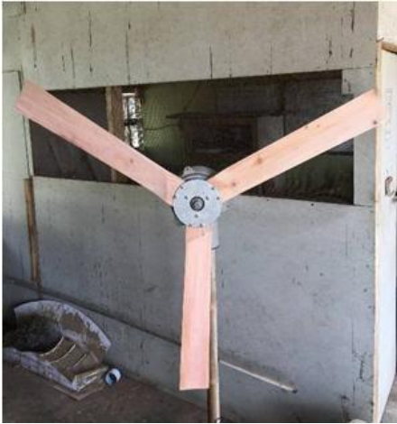
Figure 15. Balance testing process on the blade
