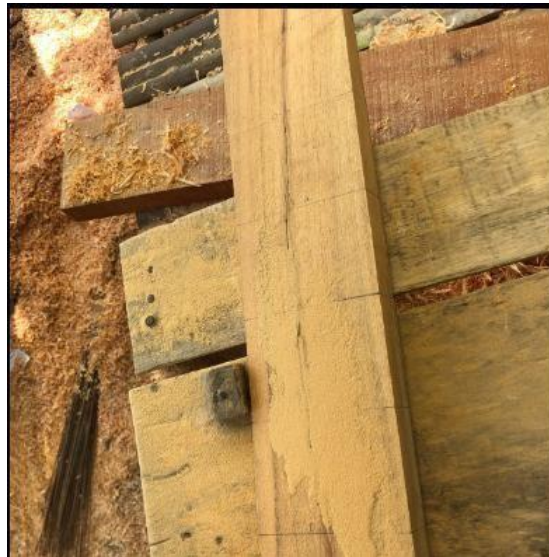
Figure 12. Making guide lines in twist formation
