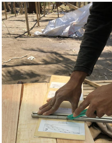
Figure 10. Process of cutting the template that has been printed out on plywood
