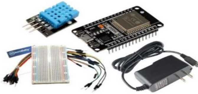
Figure 1. Hardware Components and Circuit Setup (ESP32, DHT11, Breadboard, and Supporting Devices)
