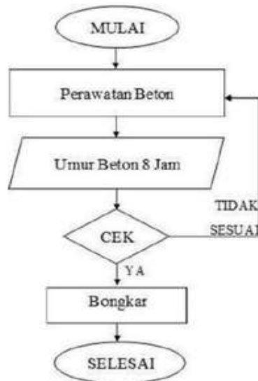
Figure 8. Flowchart of Column Formwork Dismantling
